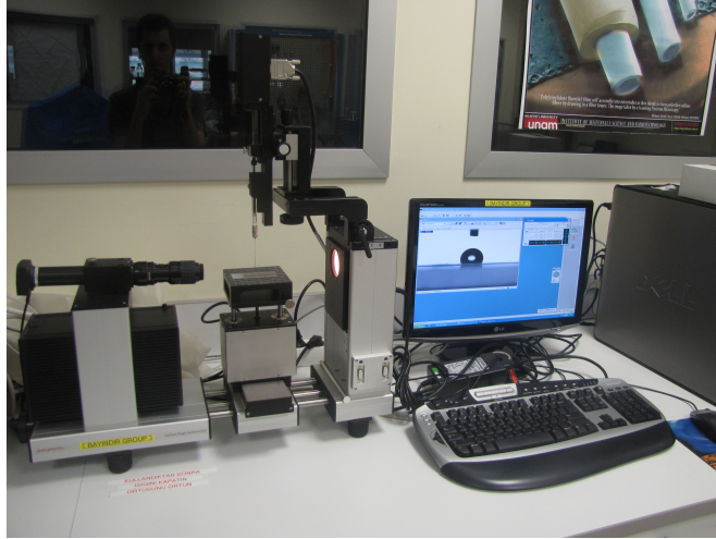
Figure 4.6: Contact angle setup gives an edge to analyse hydrophobic feature of the samples.
